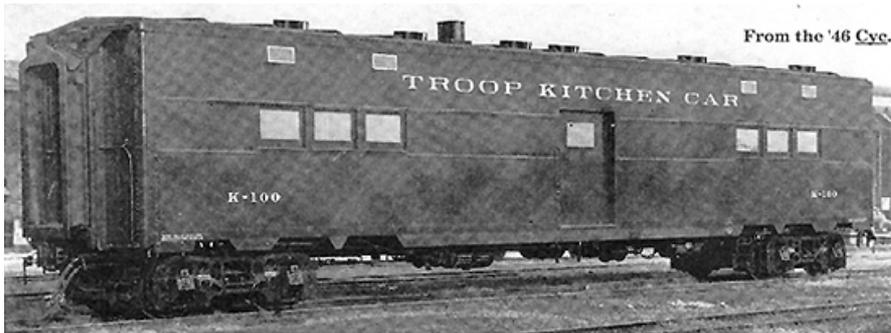
Fig. 5.412—Troop Kitchen Car based on A.A.R. standard, 50 ft. 6 in. box car design.
